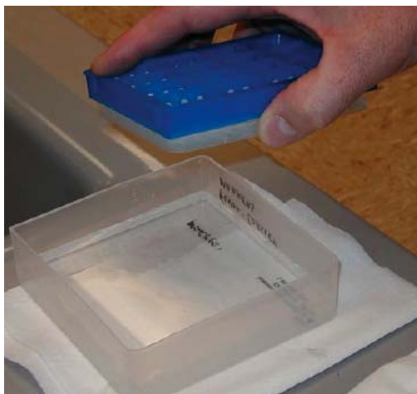
Figure 2. Ensure the plate is kept inverted during the blotting process.
